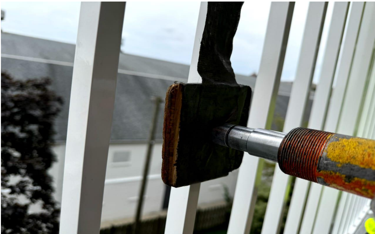
Photograph 10: Showing outward load application at the infill picket panel mid-section
