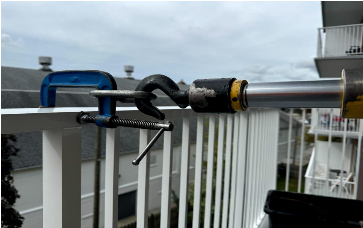
Photograph 5: Showing inward load application at the top of an intermediate post
