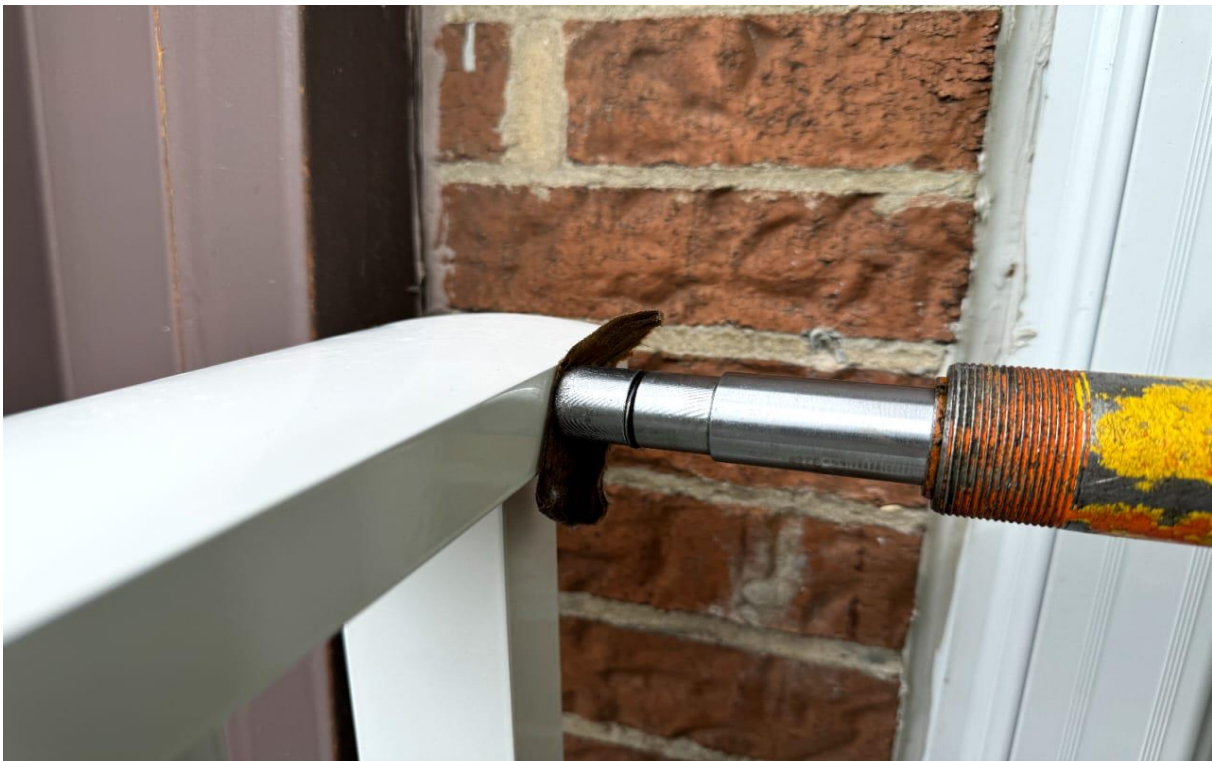
Photograph 6: Showing outward load application at the top of an end-post
