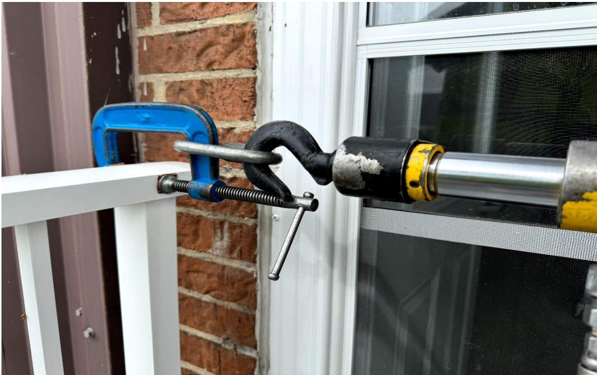
Photograph 7: Showing inward load application at the top of an end-post
