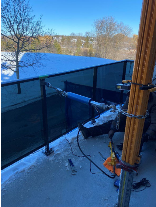
Photograph No. 5 Intermediate Post Inward Load Application (Top)
