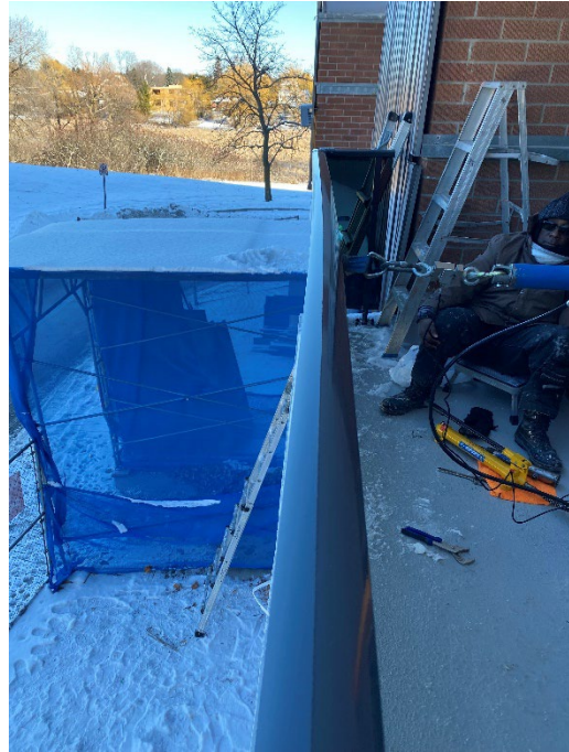
Photograph No. 6 Intermediate Post Inward Load deflection (Top)
