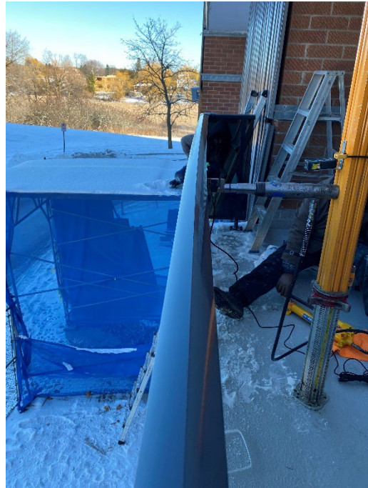
Photograph No. 4 Intermediate Post Outward Load Deflection
