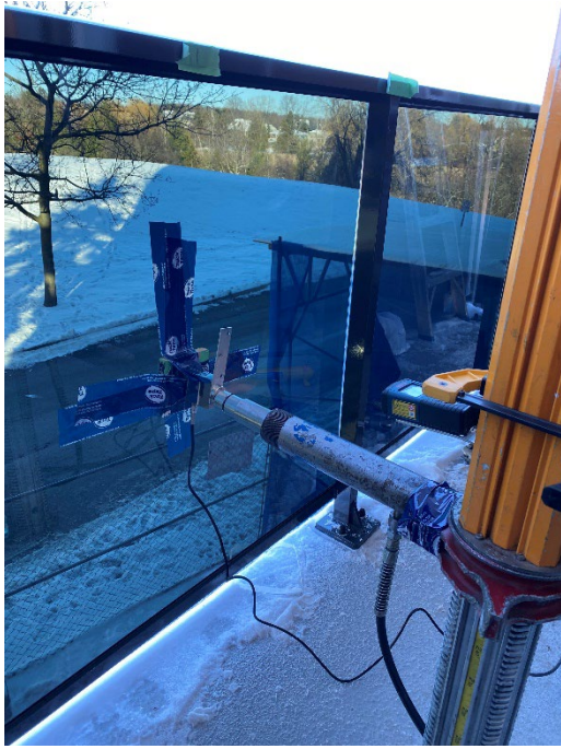
Photograph No. 9 Tempered Glass Mid-Section Outward Load Application
